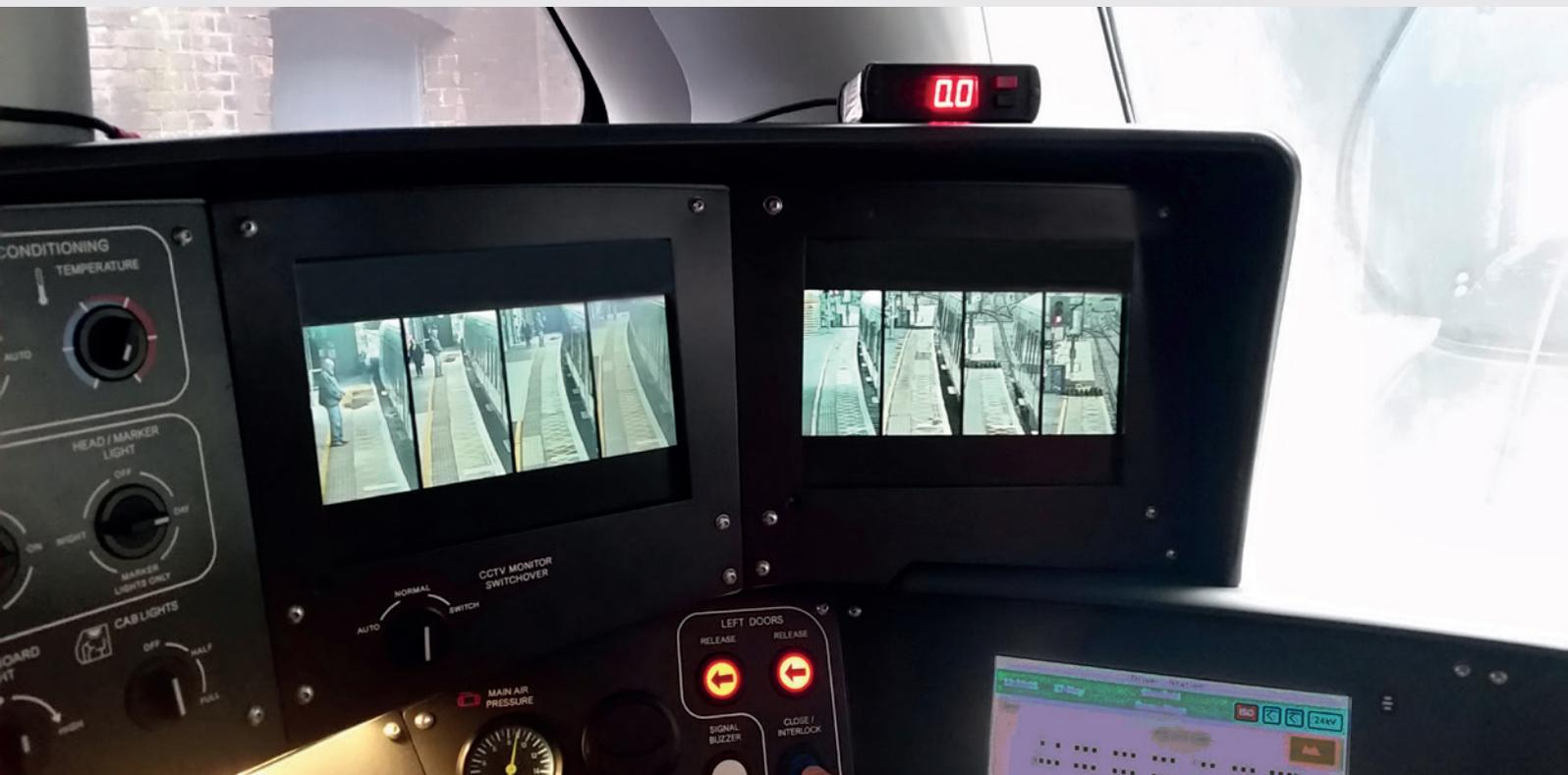
**KeLink1000™** is a Driver Only Operation CCTV system for safe departure and the enhancement of customer safety.
