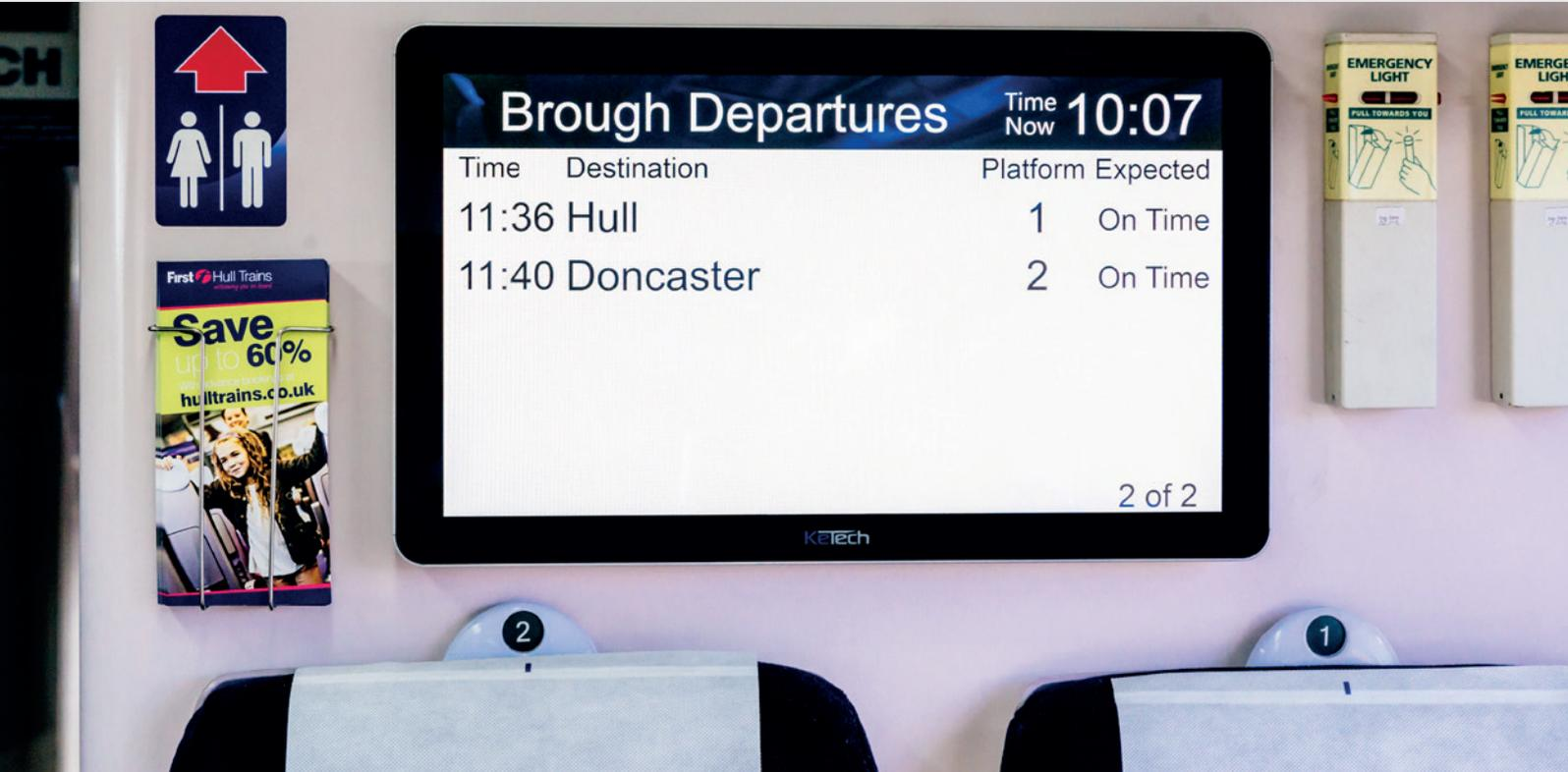
The scope also incorporated the introduction of new hardware in the form of intelligent 21" TFT HD displays with simplicity of architecture and fitment requirements that receive the live, real-time data via Wi-Fi, negating the need for through train wiring. This made the unit suitable for installation on both existing and new rolling stock and provided a truly cost-effective implementation.
